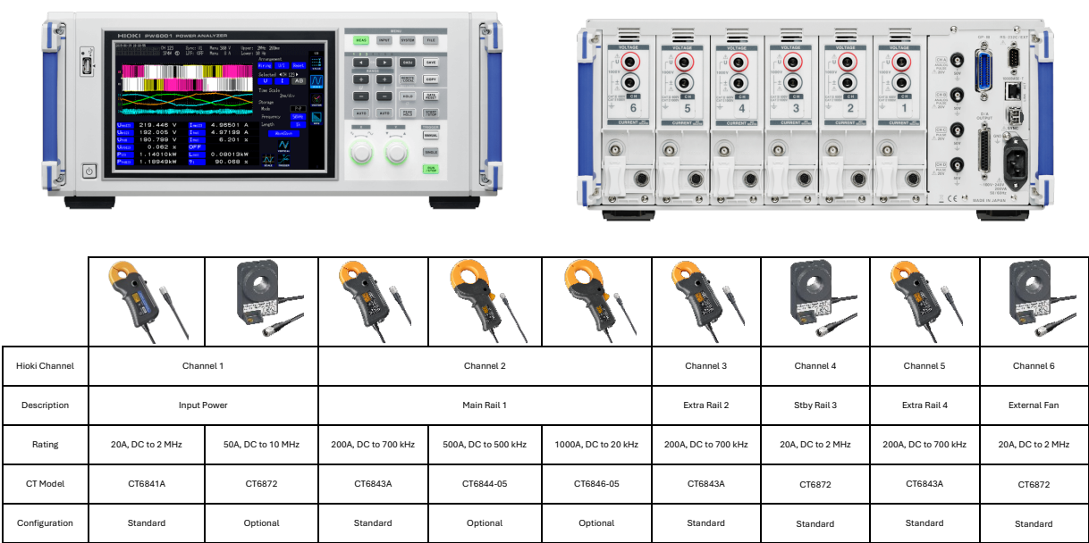
Figure 7: Hioki PW6001-16 Power Analyzer and Current Transformer Sensors
