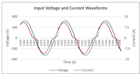
Input AC Current Waveform (ITHD = 17.82%, 50% Load)
