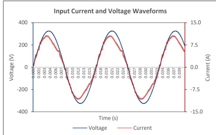
Input AC Current Waveform (ITHD = 7.48%, 50% Load)
