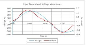
Input AC Current Waveform (ITHD = 19.45%, 50% Load)
