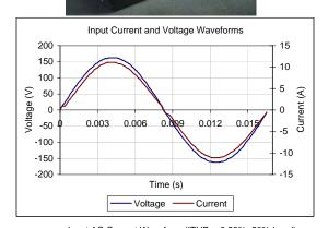
Input AC Current Waveform (ITHD = 6.53%, 50% Load)
