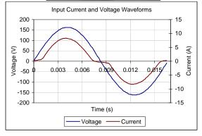
Input AC Current Waveform (ITHD = 26.33%, 50% Load)
