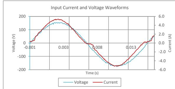
Input AC Current Waveform (ITHD = 11.7%, 50% Load)
