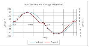
Input AC Current Waveform (ITHD = 13.191%, 50% Load)
