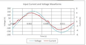
Input AC Current Waveform (ITHD = 6.96%, 50% Load)
