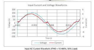
Note: All measurements were taken with input voltage at 115 V nominal at 60 Hz.
