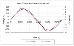
Input AC Current Waveform (ITHD = 9.38%, 50% Load)
