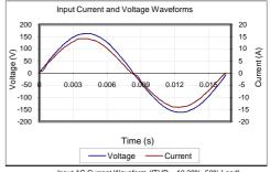
Input AC Current Waveform (ITHD = 10.38%, 50% Load)
