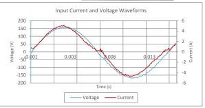
Input AC Current Waveform (ITHD = 10.66%, 50% Load)
