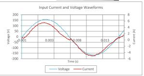
Input AC Current Waveform (ITHD = 12.32%, 50% Load)
