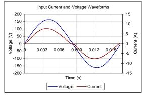
Input AC Current Waveform (ITHD = 12.14%, 50% Load)
