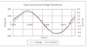
Input AC Current Waveform (ITHD = 3.95%, 50% Load)
