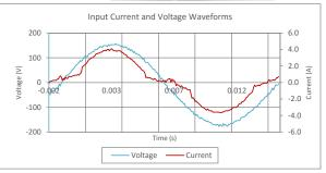
Input AC Current Waveform (ITHD = 24.44%, 50% Load)
