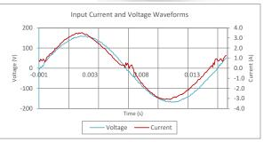
Input AC Current Waveform (ITHD = 9.53%, 50% Load)
