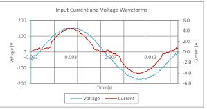
Input AC Current Waveform (ITHD = 25.29%, 50% Load)
