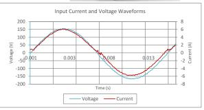
Input AC Current Waveform (ITHD = 5.614%, 50% Load)
