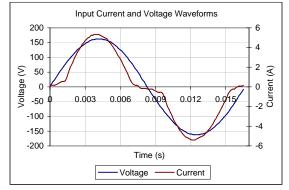
Input AC Current Waveform (ITHD = 27.58%, 50% Load)
