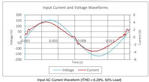
Note: All measurements were taken with input voltage at 115 V nominal at 60 Hz.
