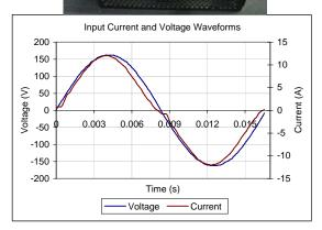
Input AC Current Waveform (ITHD = 12.2%, 50% Load)
