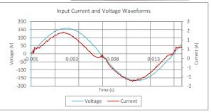
Input AC Current Waveform (ITHD = 9.55%, 50% Load)
