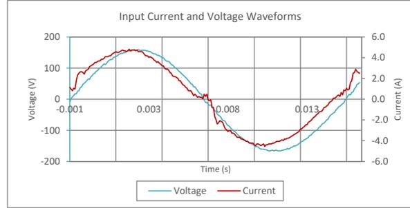
Input AC Current Waveform (ITHD = 7.04%, 50% Load)
