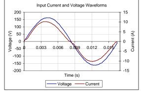
Input AC Current Waveform (ITHD = 8.89%, 50% Load)
