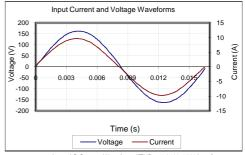
Input AC Current Waveform (ITHD = 5.05%, 50% Load)
