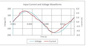
Input AC Current Waveform (ITHD = 12.83%, 50% Load)
