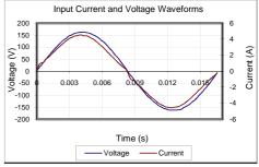
Input AC Current Waveform (ITHD = 8.12%, 50% Load)
