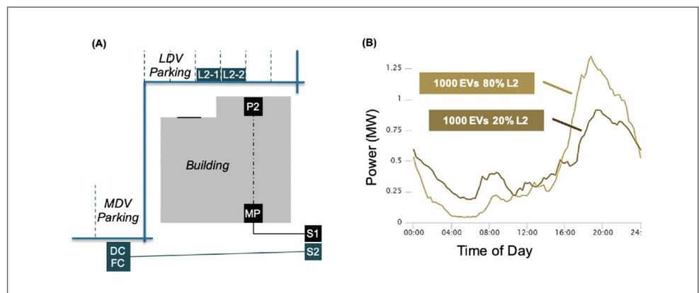
Figure 7. Optimizing site layouts (A) and load comparison of Level 1 dominant versus Level 2 dominant charging in multifamily (B)
