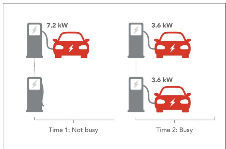
Figure 8. Illustration of automated load management
