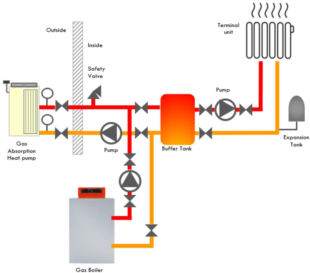
Figure 10: Sample schematic of a GAHP applied to a hot water system
